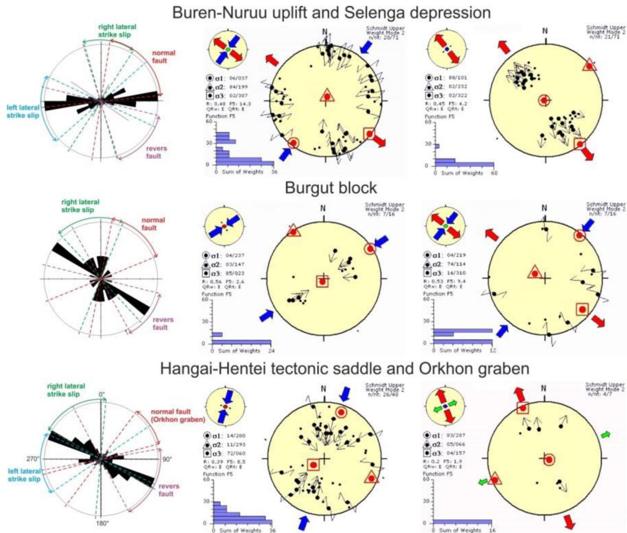
Figure 2: Faults kinematics and the results of the Late Cenozoic crustal stress reconstruction of the Central Mongolia. Left column – rose-diagrams of the active fault directions; central column – reconstructions of the prevailing stress tensor; right column – reconstructions of the secondary stress tensor.
